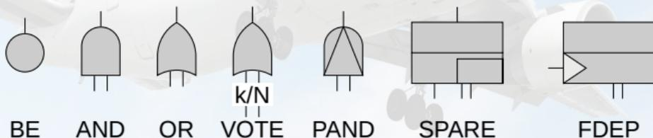
Images of the elements in a dynamic fault tree
